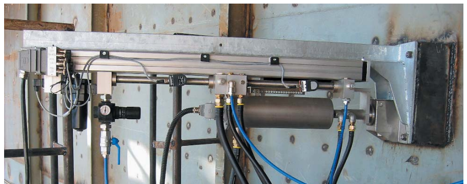
Combustion chamber sensor with retraction unit (water-cooled)
